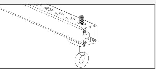
Fasten the hardware securely and repeat to create two points of contact from which the fixture will hang.
