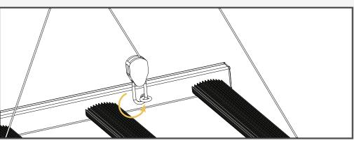
Hook the ratchet pulley end with carabiner clip into the hanging ring on the fixture. It's helpful to have another person hold the fixture while the other uses the extra length of the cord to adjust the fixture's height.
