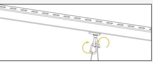
Hook the carabiner clips into the eyebolt with the ratchet pulley end hanging freely.
