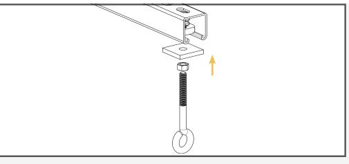
Position an eyebolt, matching nut, square washer plate, and spring nut under a channel as pictured. Note: Spring nuts with an eyebolt can also be used in this fashion.
