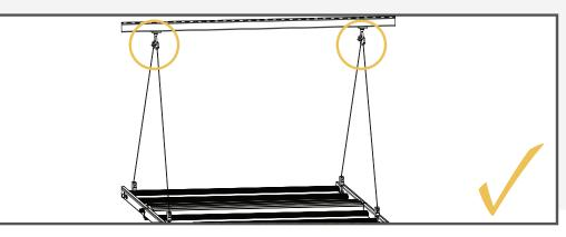
The Pisces fixture is best to hang by two or four points of contact.
