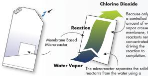
Because only a controlled amount of wate vapor crosses the membrane, the reactants remain concentrated. driving the completion. reaction-controlling membrane.
