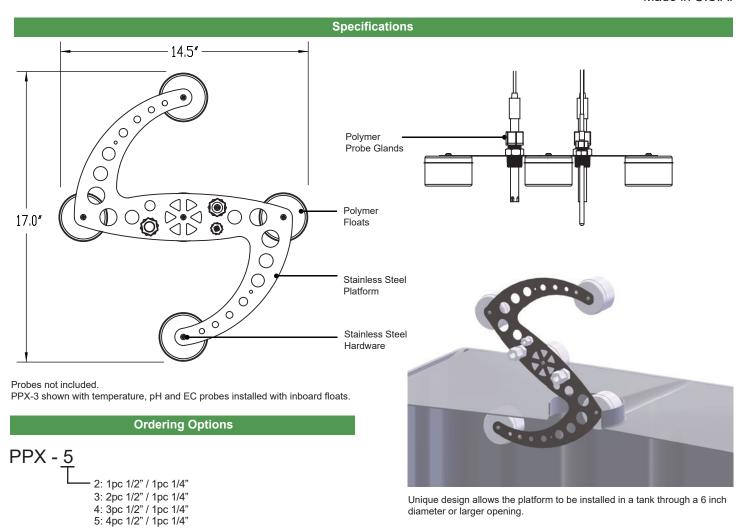
All models include four floats and can be configured for inboard or outboard mounting.
