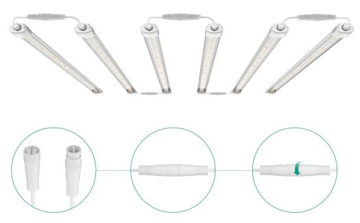
To connect the power cord, align the terminals of the cord, plug in and twist to secure.
