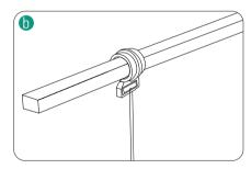
Hang the lamp on the pole using the hook of the hanging rope.
