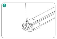
Attach the hanging rope to the hook on the light bar.
