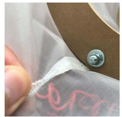
Use the staple gun to fix one end first. Adjust your staple gun to gain a perfect insert depth.
