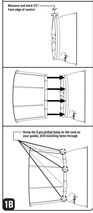
• Secure the cone to the venturi using (5) 5/16"-18x1" Phillips Truss Screws, (5) 5/16" x 1.25" OD Flat Washers, and (5) 5/16"-18 Nylock Flange Nuts.
