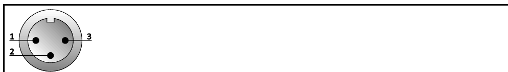
Pin assignment (front view)
