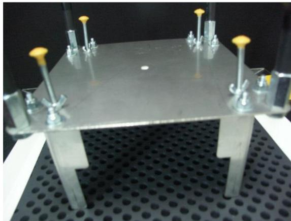
There is a wing nut underneath acting as a lock. The head of the screw is the adjustment mechanism. No tools are necessary, you do not need to turn the cradle upside down. Once you loosen the wing nut, the height adjustment screw spins freely and easily.
