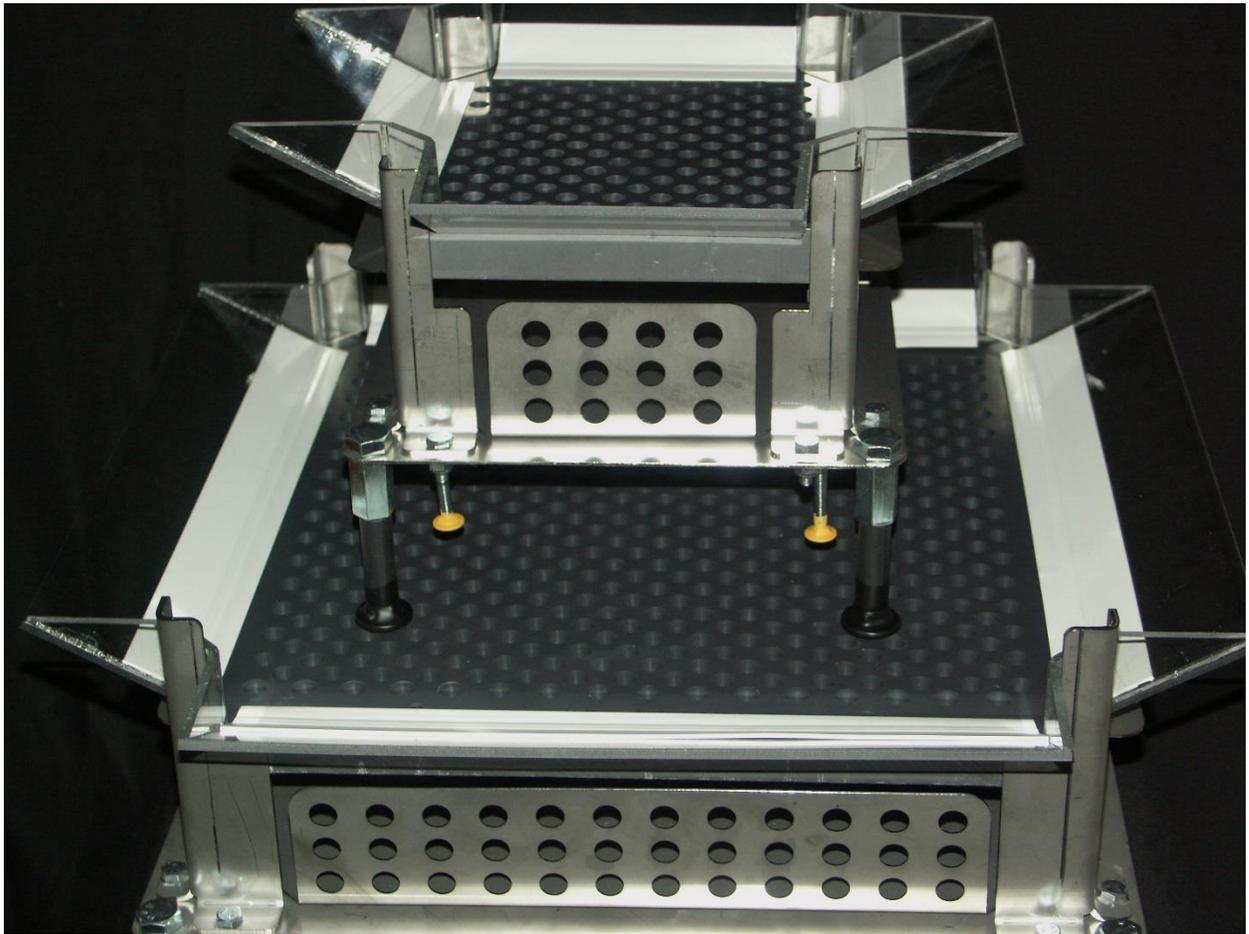
The plastic funnel provides a backstop so you can be a little more assertive when working your feedstock towards the edges and corners. The seal helps keep spillage to a minimum.
