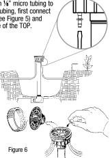
stake to end of the micro tubing and add a bug plug at the end of micro tubing. A bug plug prevents insects from crawling into the tubing, which they sometimes do to lay their eggs. The bug plug will still allow water to trickle out for the plants.
