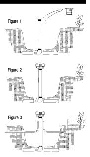
4. Remove the cover and the Mini-Disk filter. Attach ¼" micro tubing to the outlet side (see Figure 4). If using ¼" micro tubing, first connect a ¼" converter barb onto the ¼" micro tubing (see Figure 5) and then insert the converter barb into the outlet side of the TOP.
