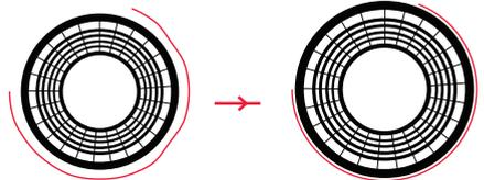
As soon as full contact between drum and shear band is achieved, release the tension knob.
