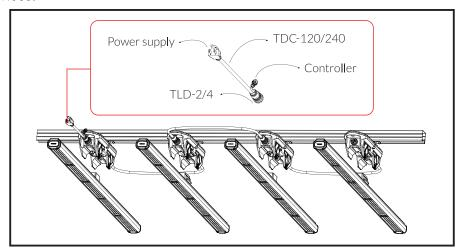
5. Next install the LED bars onto the drivers. Pay attention to the alignment & orientation of the male plug on the LED bar with the female socket on the driver. They must be properly aligned. Apply pressure on the LED bar until you hear a "click" sound confirming it is fully inserted. Ensure each LED bar is inserted fully into the Driver.
