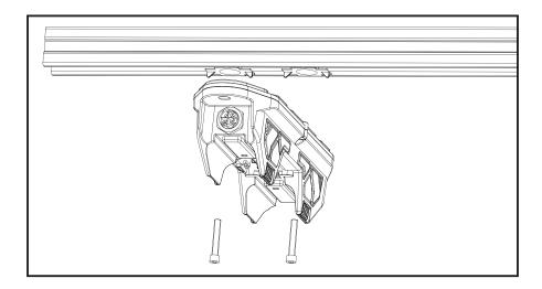
2.Attach the ThinkGrow Light Driver (TLD) to the C-channel steel using the Hex Socket Head Cap Screws.
