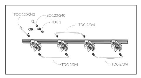
4. To set up the daisy chain configuration, first connect the TDC-120/240 or EC-120/240 and TDC-1 to the input port of the first driver. Users can use an ECS-9 cable to connect the split head of the TDC-120/240 to the controller. After that, start the daisy chain by using the TDC-2/3/4 based on the required cable length. Finally, ensure to plug the TDC-120/240 cable into a power socket to provide the necessary power supply for the connected devices.
