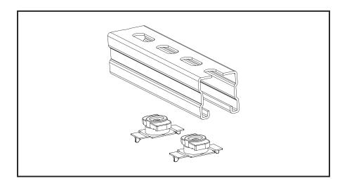
1.Position and install the MQM unistrut nuts securely into the steel C-Channel. Slide them to the correct location to achieve the spacing desired between each LED driver. Twist them 90' counter-clockwise to lock the unistrut nuts in place.
