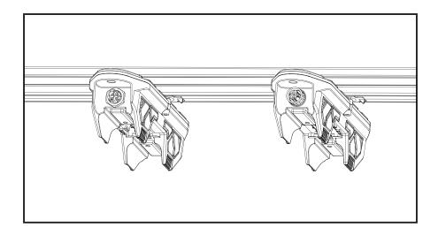
3.Ensure that the drivers are installed in an alternating pattern so that the male / female TDC cables will match up to the correct connection on the end of the Model One Drivers.
