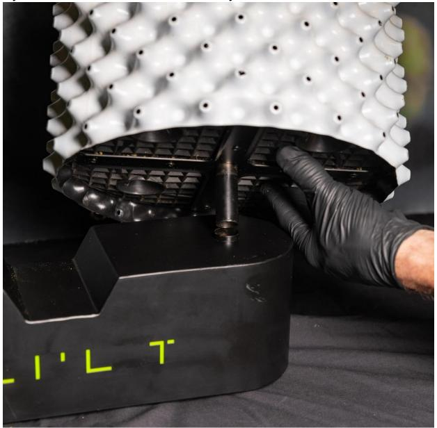
1. Lay motor down on back feet. Insert shaft into motor housing. Slowly turn cylinder clockwise until shaft drops onto receiver pin. Once shaft drops on to receiver pin, seat cylinder drum firmly in place. Cylinder is now ready for loading and trim operatio
