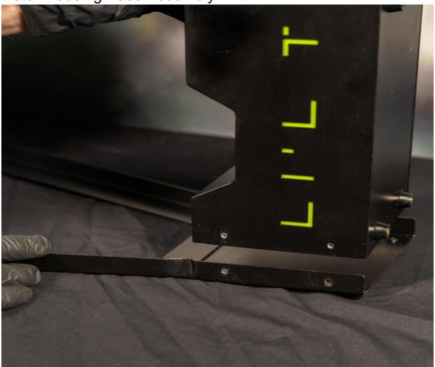
1. Lineup holes in triangle base with holes in bottom of motor housing..
