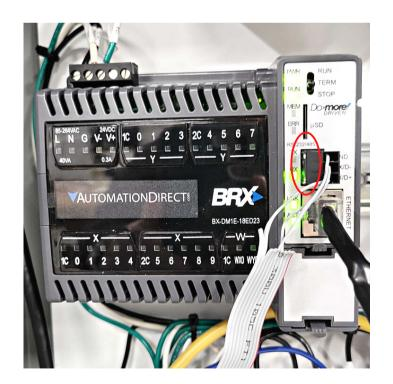
To begin data logging, access the PLC in the back of the machine. Insert a MicroSD card into the slot (see image). Once the MicroSD card is inserted, a button will pop-up on the screen with a prompt to save current weights. It's recommended to backup data once a week for record-keeping.
