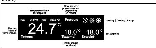
Home screen: Temperature control is inactive or an error message is displayed
