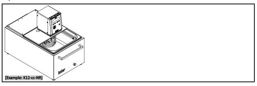
Note the volume displacement caused by a sample (e.g. Erlenmeyer flask). Place your sample into the empty bath. Only then fill in a sufficient amount of temperature control medium. Also note that the level of the temperature control medium drops when you remove the sample. This may cause a safety shutdown (low level protection) during an enabled thermoregulation. Therefore, switch off the temperature control unit beforehand.
