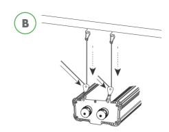
Lift the LED and attach the carabiners to pre-installed hooks from ceiling or mounting beam. The Ratchets should be installed closest to the LED (and not the ceiling).
