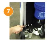
Insert the hose onto the filter barb and secure with the clamp.
