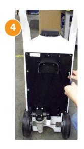
Re-attach the black plate back onto the DosaCart by installing eight screws around the plate except for the top two screws (these will be used for the crash bar, see step 9).
