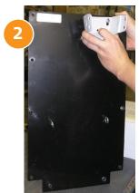
Attach the 14 GPM Dosatron unit bracket on the eyebolts, with the two screws and two nylon locking nuts provided in the hardware bag.
