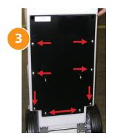
Attach the plate back onto the DosaCart by installing eight screws around the plate except for the top two screws (these will be used for the crash bar, see step 7).
