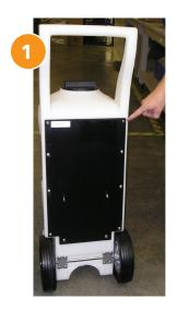
Remove the 10 screws from the back plate, to remove from the back of the DosaCart.
