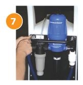
Attach the crash bar into place using the remaining two screws.
