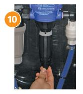
Remove the hose nut from the unit. Insert the pickup hose through the nut and attach to the barb at the bottom of the unit. Tighten the hose nut back to the unit.
