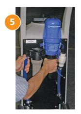
Attach the Dosatron unit and Quick Hook-Up Kit assembly onto the unit bracket.
