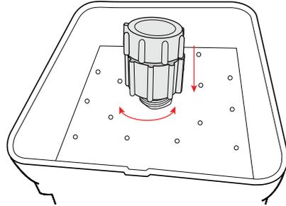
10. This water diffuser is optional. It screws on top of drain Module. **IT MUST BE REMOVED AFTER 3 weeks** this will allow roots to get optimum water.
