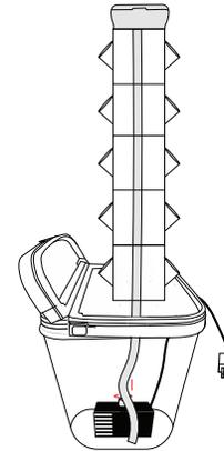
7. Place drain module on top of assembled tower and feed tubing down through modules.
