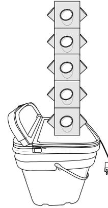
5. Build the tower, stacking grow modules on top of one another (If tower is more than 6 Modules, IT is strongly recommended to GLUE them together using standard, food safe PVC glue.
