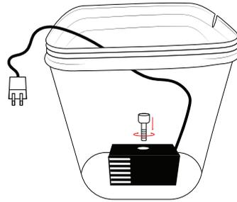
2. Attach correct nozzle fitting for tubing in the pump box. Seat pump in center of nutrient pail and adhere the suction cups to pail bottom.
