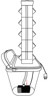
9. Attach tubing onto pump nozzle that you have attached to the pump earlier then add water and nutrients as needed. Fill nutrient pail up to 1" below top. Mix nutrients in a separate small water container. Making sure all are dissolved.. Add to nutrient pail.
