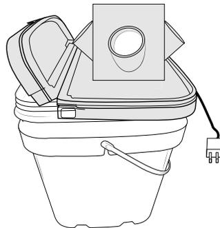
4. Snap the lid onto the nutrient pail; hinged front end accesses the pump. The larger part of the lid snaps over the pail notch. Make sure large part of the lid is snapped on tight. Leave hinged end open. DO NOT pull the side tabs on the lid.
