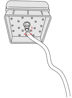
6. Carefully twist the tubing onto the barb on under-side (bottom) of the drain module until it is half way inserted in the tubing. Hold top of barb as you GENTLY twist the tubing. \*Do NOT Force \*
