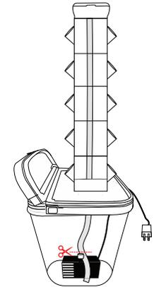
8. Pull tubing to correct length (top of Pump nozzle) and trim off excess.
