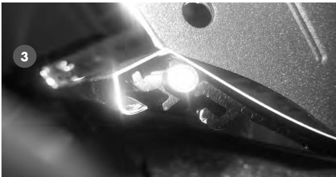
Pry end of reflector open
