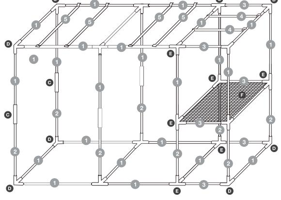
Connect the grow tent framework ensuring the poles are seated properly in the corner connectors. It may be necessary to gently twist the poles back and forth to make a secure connection.
