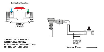
Step 4 - Glue the coupling into the line.
