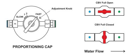
Step 9 - Turn on a sprinkler or drip zone with the closest to average gallons per minute flow rate and watch the clear fertilizer out tubing for color
