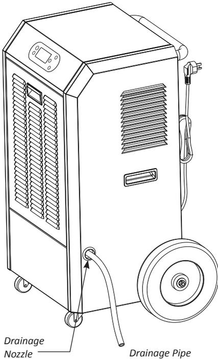
**WARNING:** Do not block the drainage hose. The end of the drainage pipe should not be higher than the outlet hole. If the drainage pipe end is higher than the outlet hole, water will not drain properly and could damage components of the unit.
