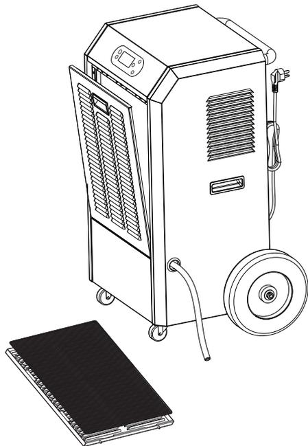
3. Remove the filter mesh out of the unit.
