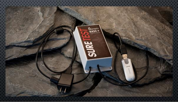
THE GROGURU BASE COMMUNICATES WITH THE GROGURU STEM + SENSORS CREATING A SYSTEM THAT CAN BE REMOTELY MONITORED WITH THE GROGURU APP.
