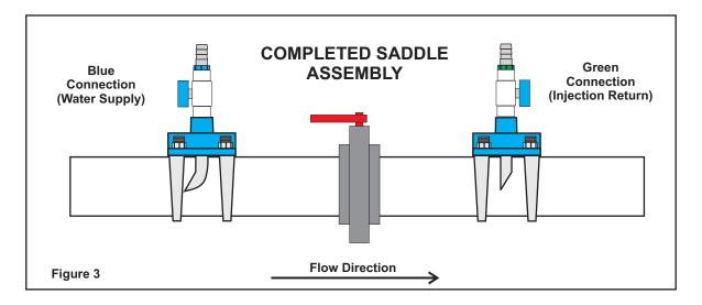
Note: A butterfly or ball valve may be required for low flow irrigation mainline to allow for throttling. This will increase the differential pressure necessary to operate the system. Contact an EZ-FLO representative for more details and calculations.
