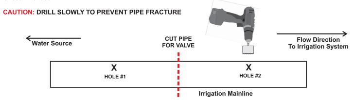
**Step 2 - Attach saddle to pipe.** The blue connection should be installed in the first drilled hole in the irrigation main line with the venturi probe opening facing into the water flow. The green connection should be installed in the second drilled hole in the irrigation main line with the venturi probe opening facing away from the water flow.
