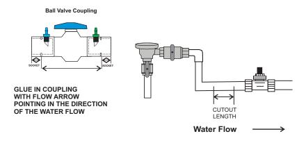
Step 4 - Glue the coupling into the line.
