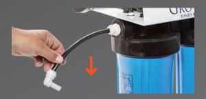
Point this tubing down into a bucket or drain, and slowly turn on the incoming water supply. Carbon dust will start pouring out. Flush KDF carbon filters for at least 20 gallons.
